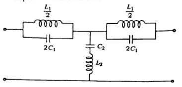
(b) Show that the characteristic impedance of following symmetrical T-section is given by  $Z_0 = \sqrt{\frac{Z_1^2}{4} + Z_1 Z_0}$ :
