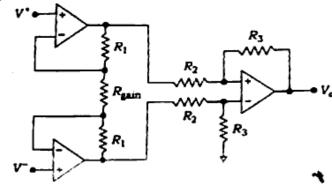
If  $R_1 = 10 \text{ k}\Omega$ ,  $R_2 = 5 \text{ k}\Omega$ ,  $R_3 = 10 \text{ k}\Omega$ and  $R_{\text{gain}} = 5 \text{ k}\Omega$ , what is the gain of the instrumentation amplifier? 7+7
