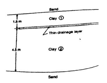
If a structure is constructed above the clay layer, how many days would be required for it to attain half the ultimate settlement? Assume that the expression  $T = \pi / 4U^2$  is applicable for the entire range of consolidation.
