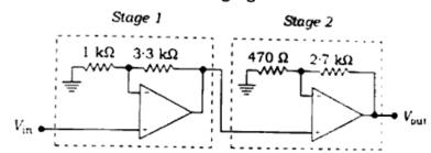
Calculate the voltage gain of this amplifier circuit  $(A_{\nu})$ :
